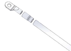
Figure 5-2 Copper terminal, heat shrink tube, and copper wire.
